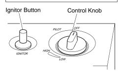
Figure 15 - Control Knob In The OFF Position
